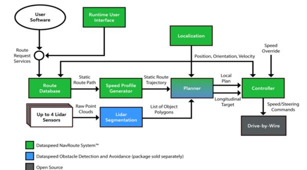
Image 3: Flow chart displaying how the NavRoute system operates.
