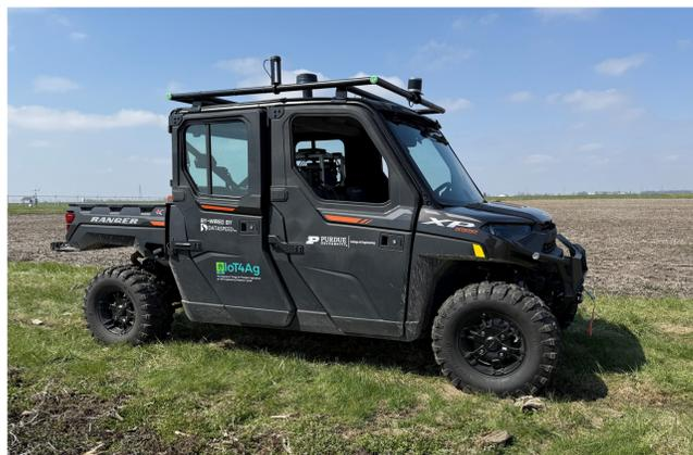
Image 1: Polaris Ranger UTV equipped with DataSpeed's autonomous drive-by-wire system
